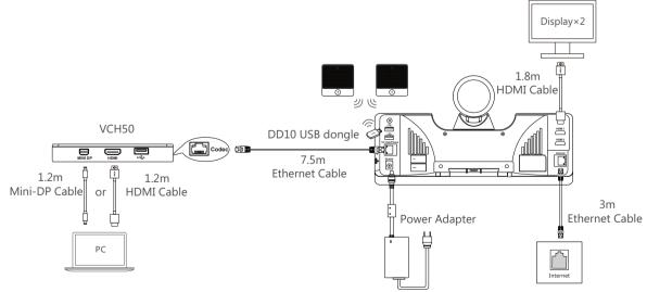
$igodoldsymbol{Q}$  The CPW90 wireless microphones and DD10 USB dongle are automatically paired from the factory.
