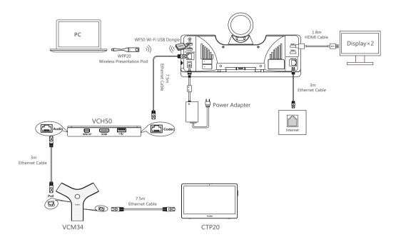
Figure 4 If you do not need the VCH50 video conferencing hub to share content, you can connect the VC Hub/Phone port on the system to the PoE port on the VCM34 directly.
